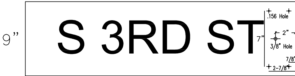
D3-1A 9x36 Copy – 6 Inch Highway Gothic Series B 3-M Hi-Intensity Silver Legend on a Hi-Intensity Green Background
