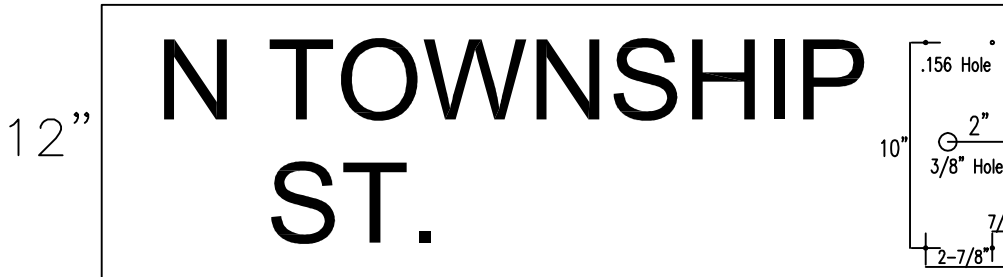
D3-3 12x36 Copy – Two Lines 4 Inch Highway Gothic Series B 3-M Hi-Intensity Silver Legend on a Hi-Intensity Green Background
