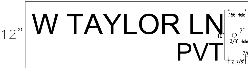
D3-3PVT 12x36 Copy – Line 1 – 6 Inch Highway Gothic Series B Line 2 – 3 Inch Highway Gothic Series B 3-M Hi-Intensity Black Legend on a Hi-Intensity Yellow Background
